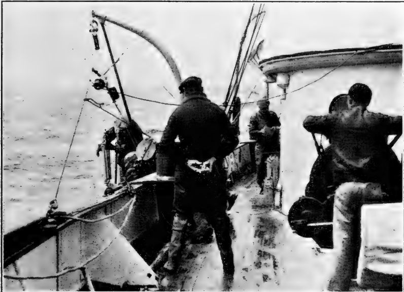
FIGURE 1.—Oceanographic work aboard the U. S. F. S. Albatross II . One of a series of Greene-Bigelow water bottles with a sample of sea water from a known depth is being brought aboard.
